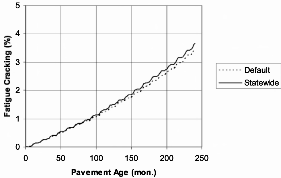
FIGURE 93. Cracking – Statewide and Default Class Distribution Factors for TTC 6
